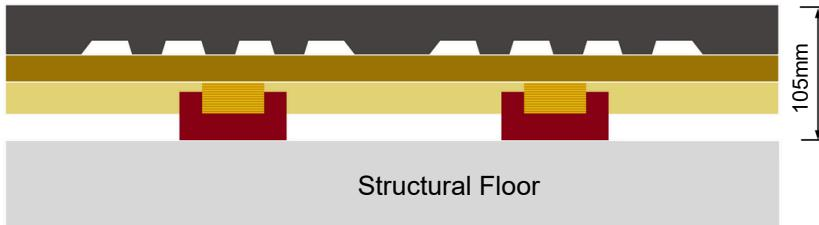
ISO-Flex 105 floor system is designed for gym applications providing a support platform for cardio fitness equipment such as treadmills and spinning bikes. This system provides impact energy absorption and acoustic isolation, reducing impact sound entering the structure.
