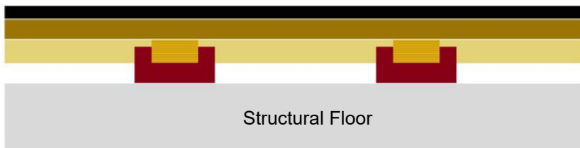
ISO-Flex 85 floor system is designed for gym applications providing a support platform for cardio fitness equipment such as treadmills and spinning bikes. This system provides impact energy absorption and acoustic isolation, reducing impact sound entering the structure.
